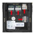
Insert the SIM/TF Card into their corresponding slots in the battery compartment.
