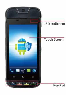
Touch screen: Displays all information needed to operate LED Indicator: Indicates system status while application generated notifications(programmable).
